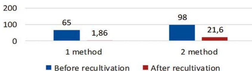
Fig. 1. The content of petroleum products in the soils of the experimental sites before and after recultivation
